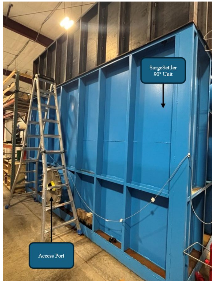
Figure 14 – SurgeSettler 90° Unit and Access Port Test Loop 2 and 3
