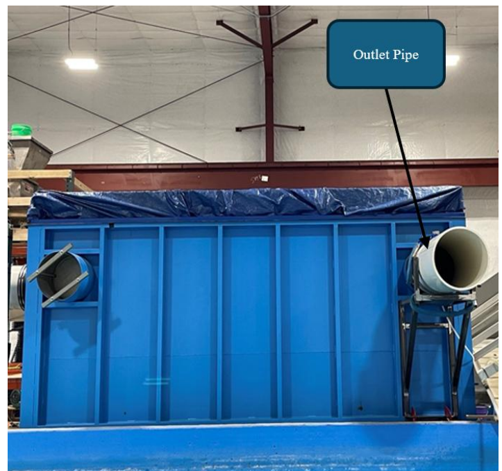
Figure 10 - Outlet Pipe Test Loop 1, Test Loop 2 and Test Loop 3
