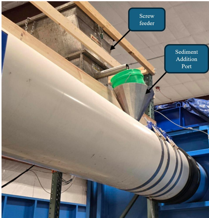
Figure 7 - Sediment Addition Port Test Loop 1, Test Loop 2 and Test Loop 3
