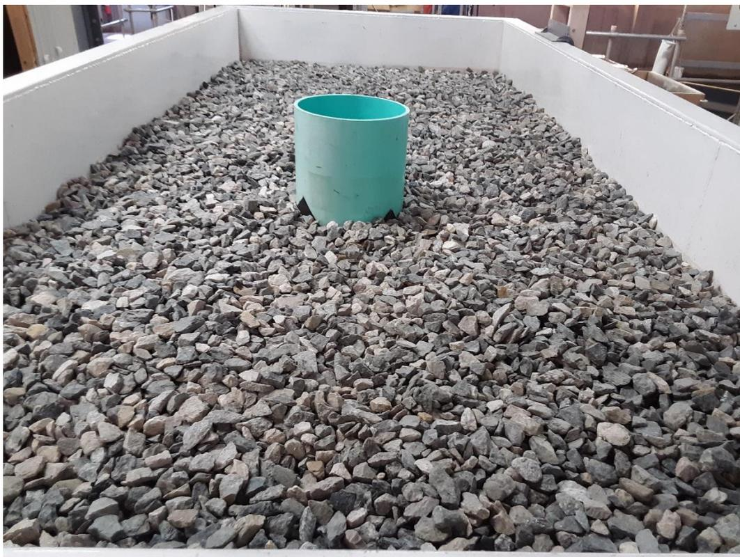
**Figure 6 Installed R-Tank Treatment Row System**
