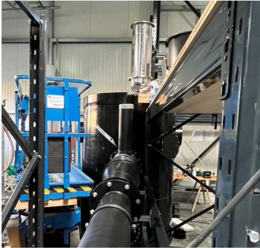
Figure 8 View of Inlet to Test Unit – Sediment Feeder and Riser
