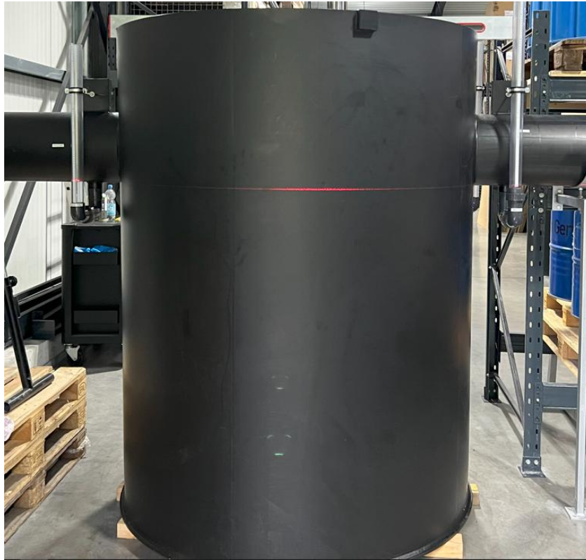
Figure 9 Test Unit Showing Inlet and Outlet Manometers
