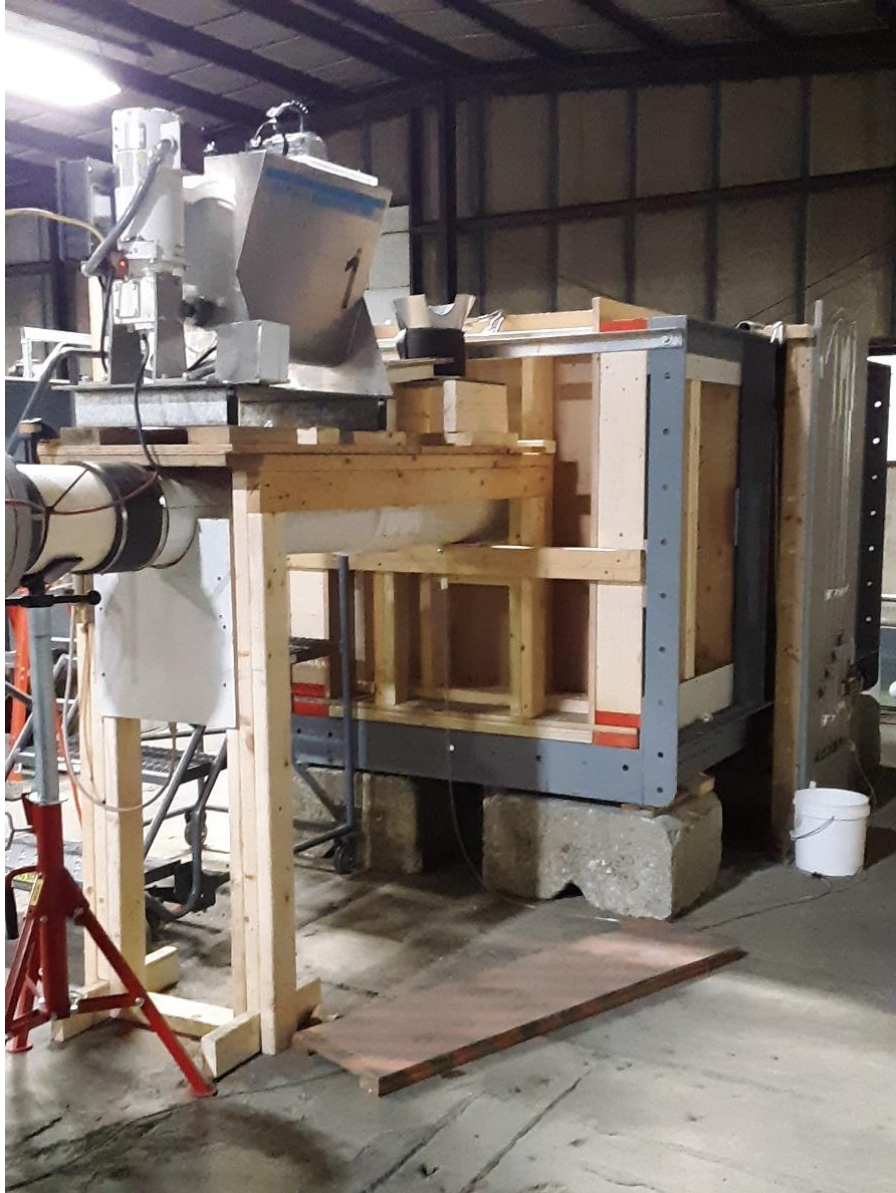
Figure 4 DryScreen® Test Unit Installed in Alden Flow Loop
