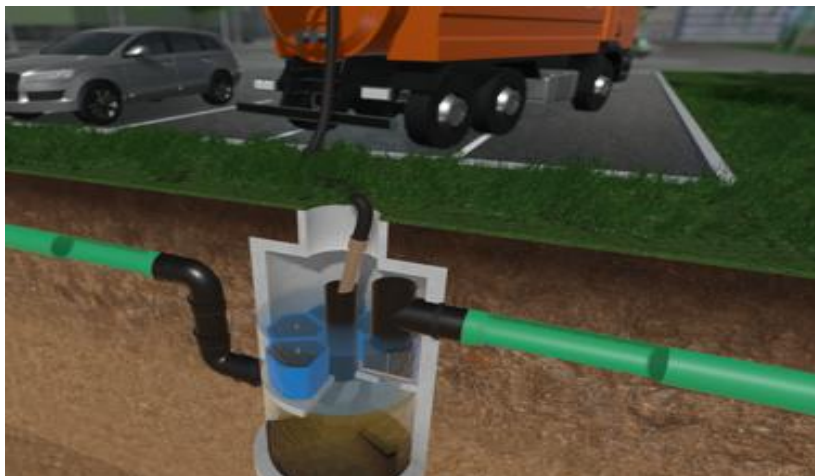
Figure 19 Emptying Out the Sediment Sump
