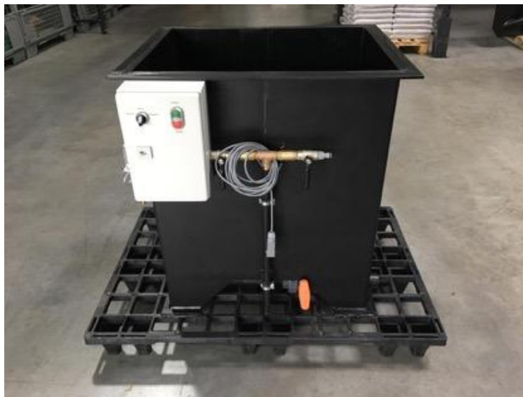
Figure 21 Mobile Filter Cleaning Unit
