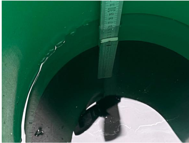
Figure 14 Fixed Ruler to Measure Driving Head
