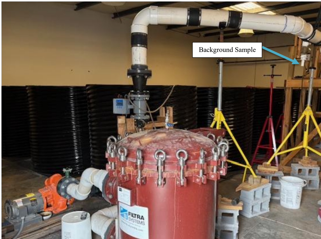
Figure 5 Background Sample Port and Test Loop Equipment Locations
