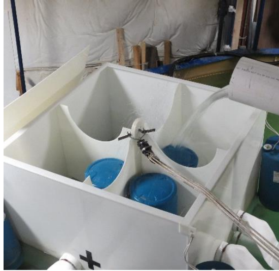
Figure 6 Effluent Sampling Location Situated above the Filter Box
